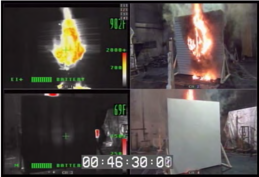
Figure 6. 44: Picture of Peak Heat Release Rate for Wall Type 8 Grill Fire
