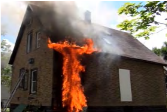
Figure 10. 22. Fire extending from a trash can into the eaves during a field experiment in Milwaukee, WI.
