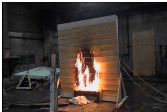
Figure 10. 12. Flame spread 2 minutes after ignition of a wood lap sided wall over polystyrene sheathing
