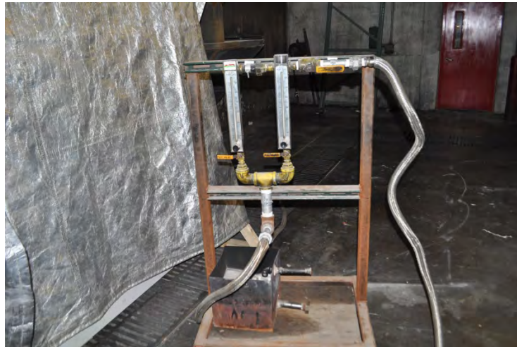
Figure 6. 5: Picture of Natural Gas Flow Controller
