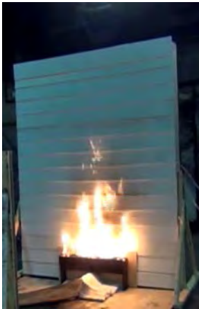
Figure 10. 8. Exp. 19 – Fiber Cement Siding
