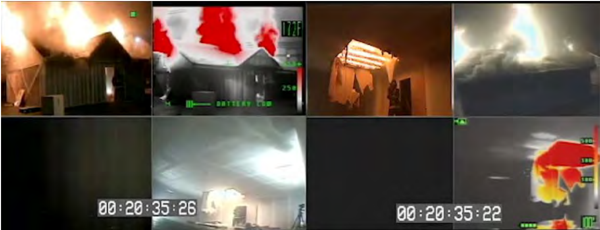
Figure 10. 26. Burning at interior ventilation opening in the ceiling during Attic Fire Experiment 2B
