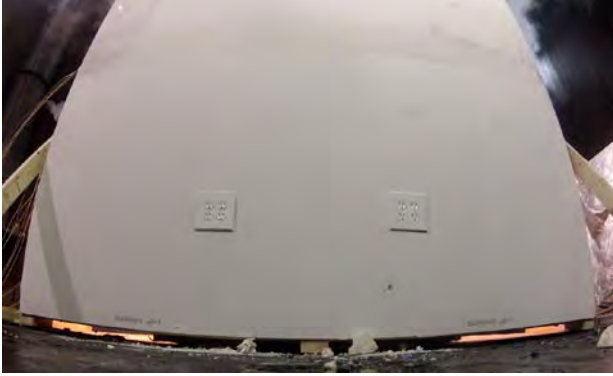
Figure 10. 24. Wall Experiment 13 before receptacle burn through
