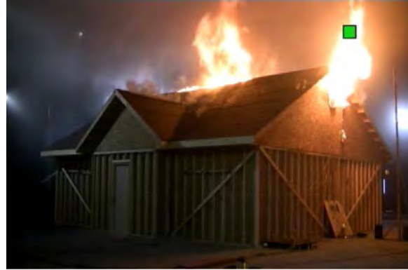
Figure 10. 30. Attic Fire Experiment 3 during peak temperatures in the attic with gable vents and roof vent opened.
