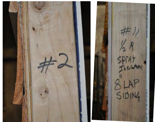
Figure 10. 4. Two wood sided wall sections with different energy efficiencies
