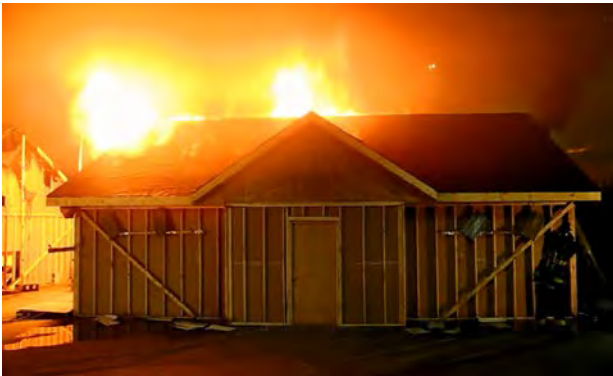
Figure 10. 36. Conditions at the start of eave attack during Attic Experiment 4
