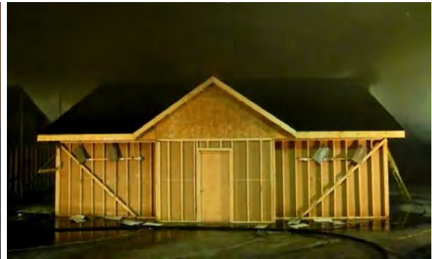
Figure 10. 37. Conditions at the end of eave attack during Attic Experiment 4
