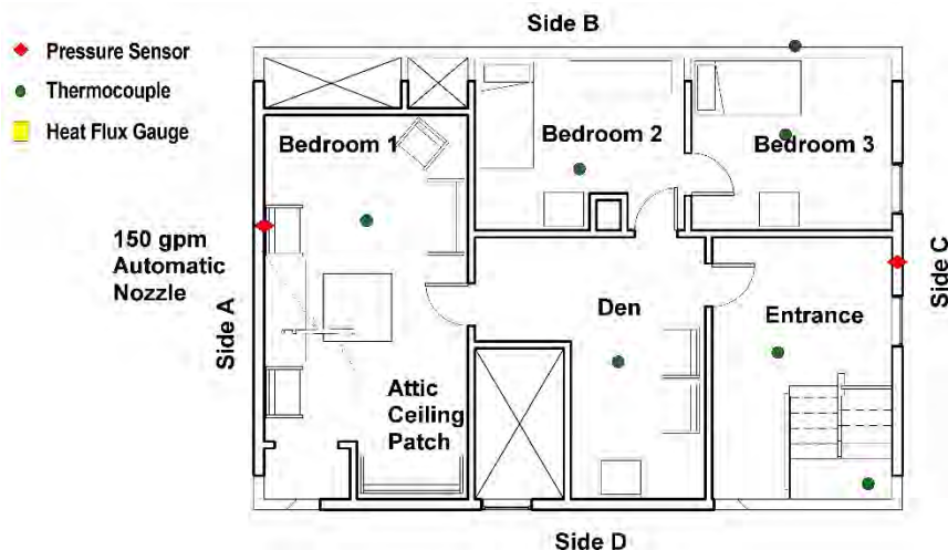
Figure 9. 10: 25th St. Attic Instrumentation
