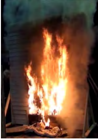
Figure 10. 5. Exp. 3 – Vinyl Siding over plywood
