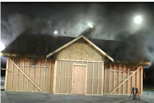
Figure 10.33. Smoke pulsing from eaves after ridge vent sealed.
