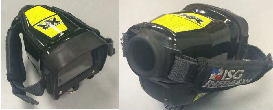
Figure 5. 7: ISG Elite XR Fire Service Thermal Imaging Camera
