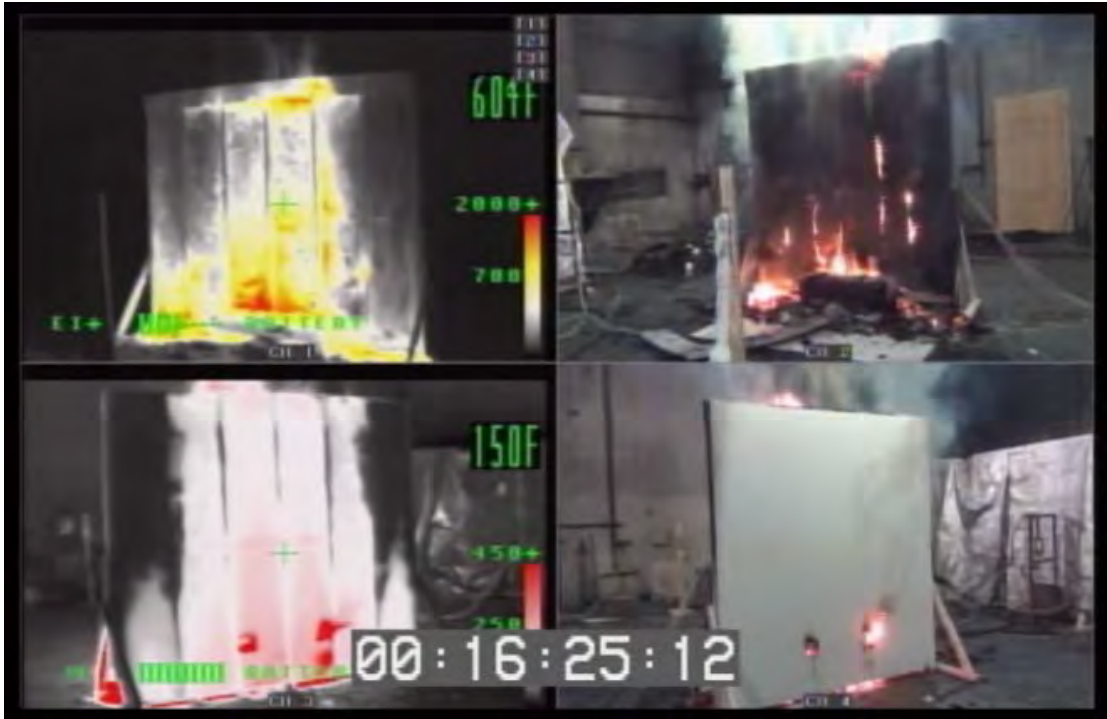
Figure 6. 46: Image of Fire out of Back Wall of Experiment 12
