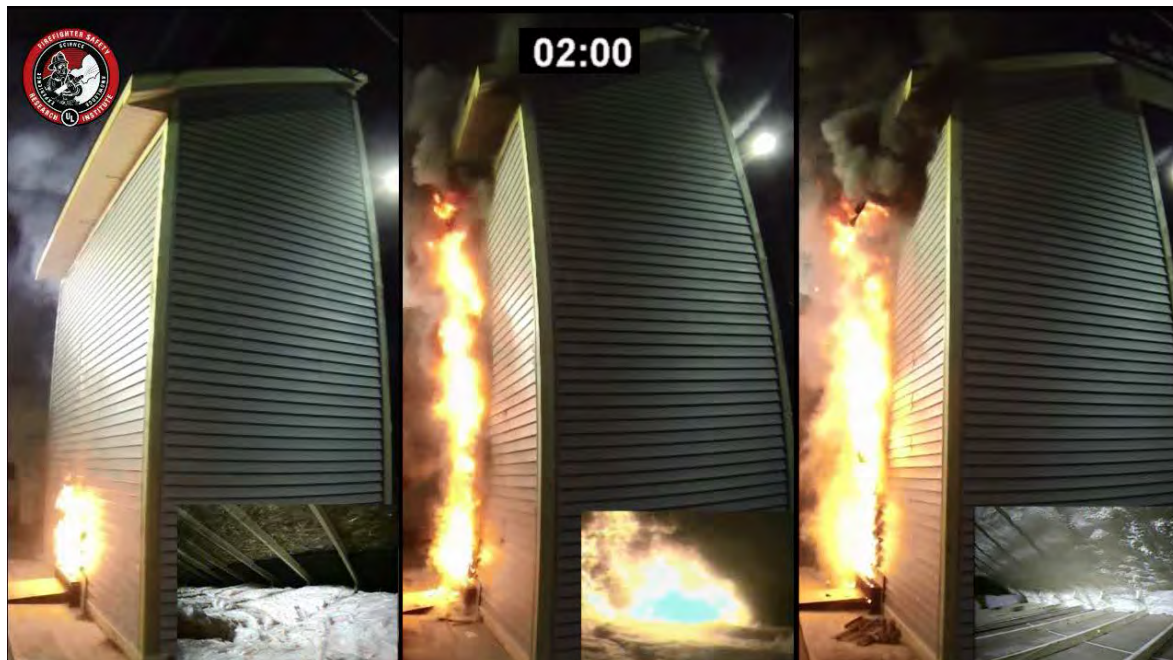
Figure 10. 13. Wall and Eave experiment as Vinyl Siding/Polystyrene Sheathing/Fiberglass Insulation system transitions to an attic fire (2 minutes after ignition)
