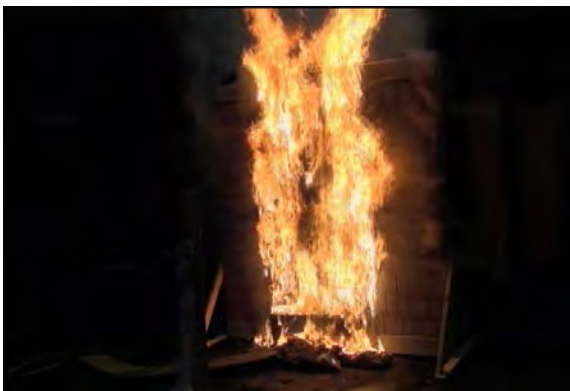
Figure 10. 11. Flame spread 2 minutes after ignition of a polypropylene shingle sided wall over polystyrene sheathing
