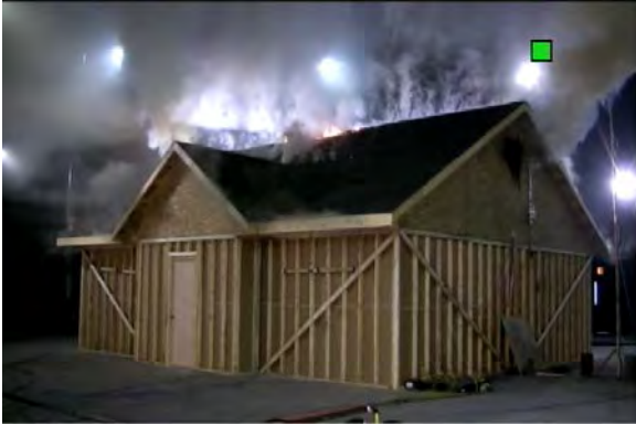
Figure 10. 29. Attic Fire Experiment 3 during peak temperatures in the attic with gable vents opened.
