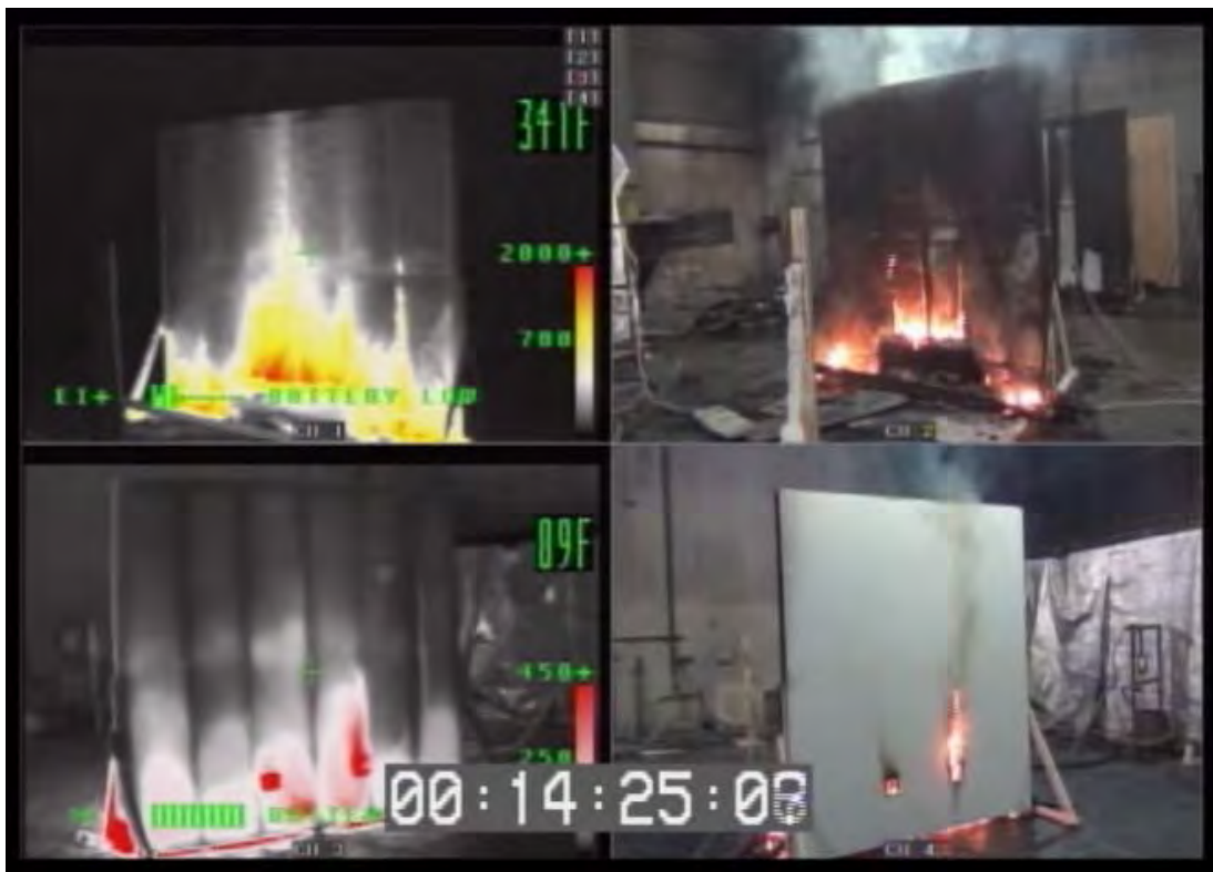
Figure 6. 47: Image of Fire out of Back Wall of Experiment 13
