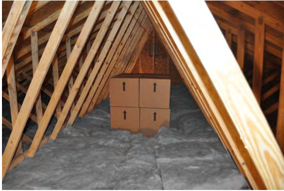
Figure 8. 9: Attic Experiment 1 Fuel Load
