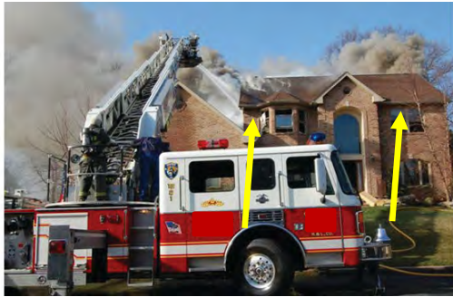
Figure 10. 41. Master stream flowing down into attic fire and not into eaves.
