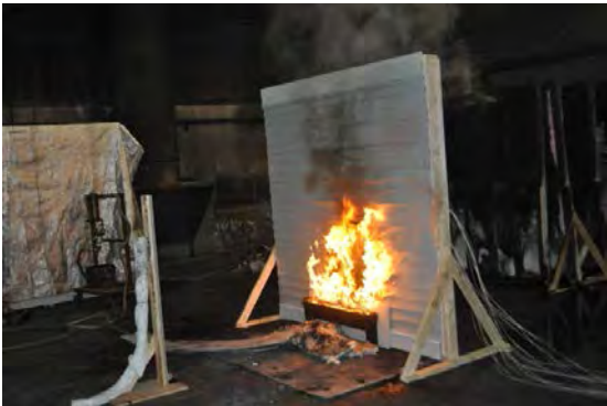
Figure 6. 3. 100 kW fire from 36 in. line burner
