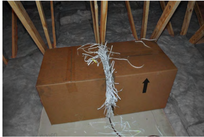
Figure 8. 11: Attic Experiment Two Box Fuel Load
