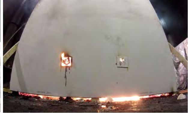
Figure 10. 25. Wall Experiment 13 after fire penetrates the receptacles
