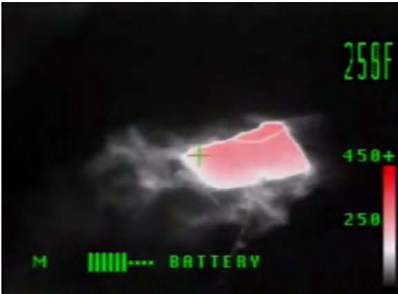
Figure 10. 27. Thermal imaging view of ceiling vent in Field Experiment 3 shortly after opening
