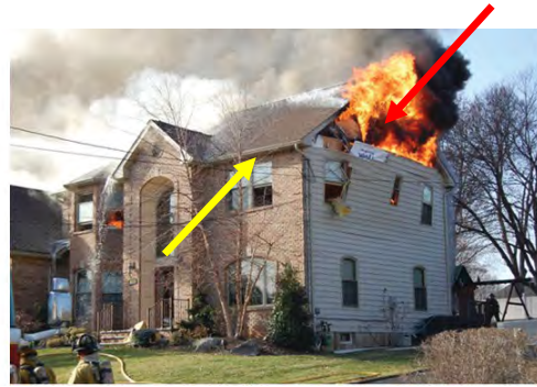
Figure 10. 42. Potential to flow water where fire is coming from instead of where fire is.
