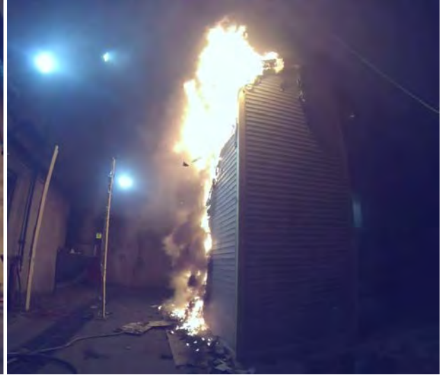
Figure 10. 21. Burning at eave line with the unvented attic (Experiment 3)
